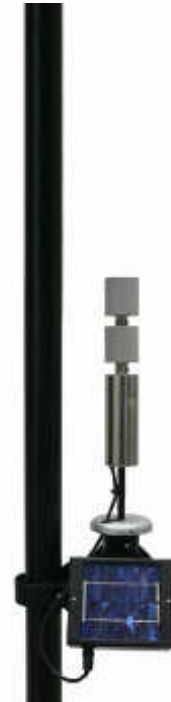
Fig. 6-3 Dual-probe configuration (internal view): EP-1B-04 mounted as secondary probe
