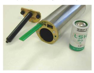
Respect polarity when replacing the battery!
