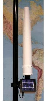
Fig. 6-4 AMB-8057 area monitor Dual-Probe configuration
