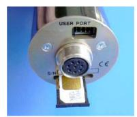
Fig. 4-3 SIM card installation
